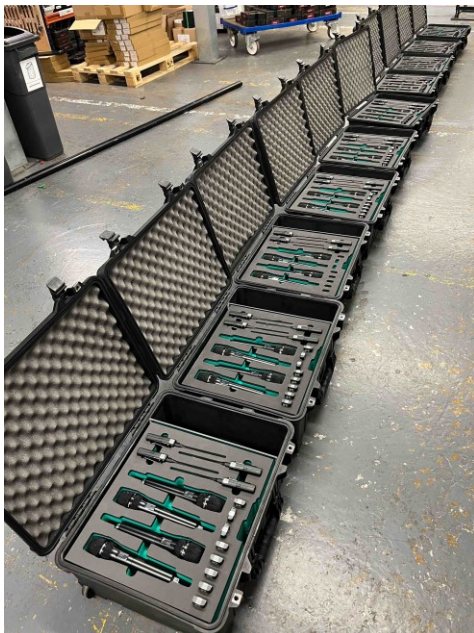
22live packed the EW-DX handheld and bodypack transmitters into ten convenient four channel sets complete with headset mics and batteries
