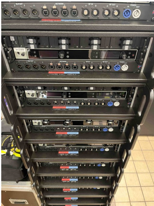
The custom-made racks, each with an EW-DX quad receiver and L 6000 charging station
